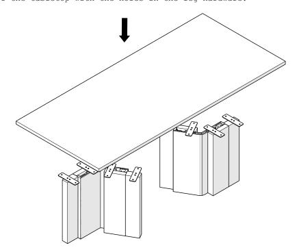
b) Insert an M8x20 Countersunk screw into each of the 16 holes where the legframe hardware meets the tabletop. Tighten firmly with an Allen Key.
